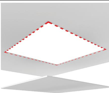
Using a plaster knife or jigsaw, cut along the marked line and remove the excess plaster.
