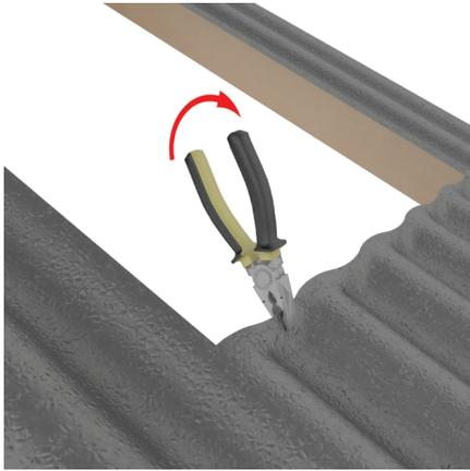
Weather up the corrugations on the low side of the cutout by folding the low spots with pliers.
