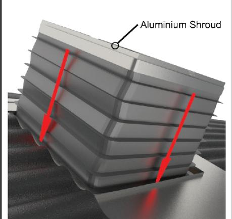
Carefully lower shroud and flexi shaft through the opening in the soaker tray.
