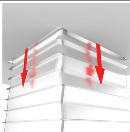
Gently pull excess flexi shaft through the ceiling opening.
