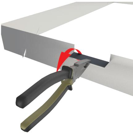
Using pliers, fold **out** the straight cut tabs on top of the aluminium shroud 90 degrees.
