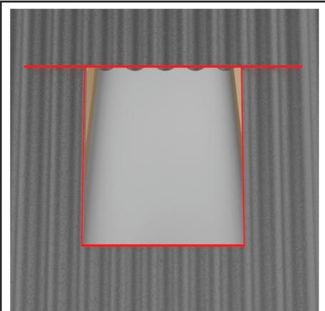
Using jigsaw, cut out marked lines and remove square roof sheet peice.
