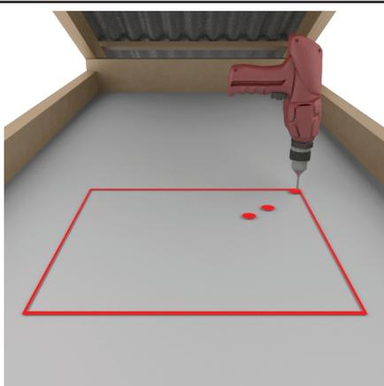
Drill a marker hole in ceiling to indicate one corner of the ceiling frame. Place two more holes to indicate direction of skylight.
