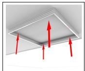
Unclip light diffuser from frame and mount frame to ceiling using fixings provided. Drill 12mm hole and feed cable through.
