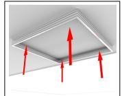
Unclip light diffuser from frame and mount frame to ceiling using fixings provided. Drill 12mm hole and feed cable through.
