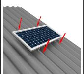
Attach brackets to the roof with screws. Seal under the screws. Run cable under ridge cap and into roof cavity.
