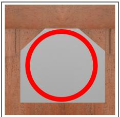
Remove several tiles from the location where Roof Vent will be positioned. You may need to cut some tiles with an angle grinder.
