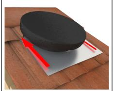
Slide the top of the soaker tray under the top row of tiles and the sides and bottom of the soaker tray sit above the tiles. The Roof Vent should now be positioned with the opening located over the hole in the tiles.
