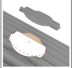
Using a jigsaw or tinsnips, cut a circle in the roofing sheet 10mm larger than the flexi shaft diameter.
