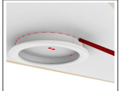
From inside the building (looking up at ceiling) locate the original hole for position ceiling ring.
