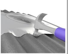
Using a hammer or rubber mallet, gently form the edges of the tray to match the roof profile.
