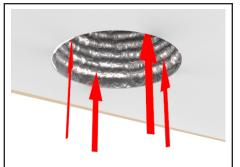
Push hanging flexi shaft back up into roof cavity.
