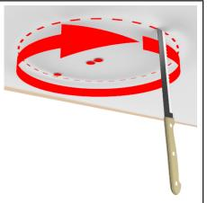
Using a plaster knife or jigsaw, cut out the plaster circle and remove.
